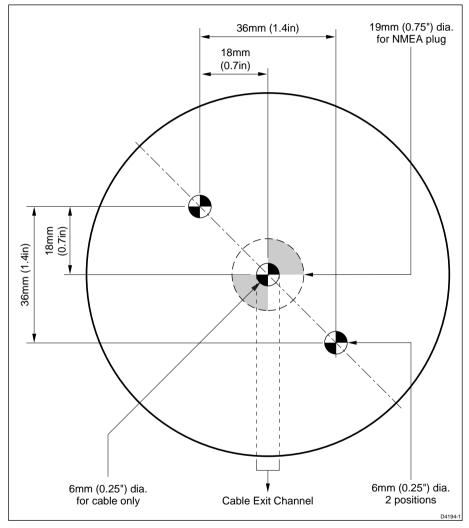
**Note:** Access to the underside of the mounting surface must be available to allow for secure fixing.
